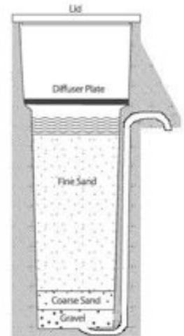
BioSand Filter Schematic
